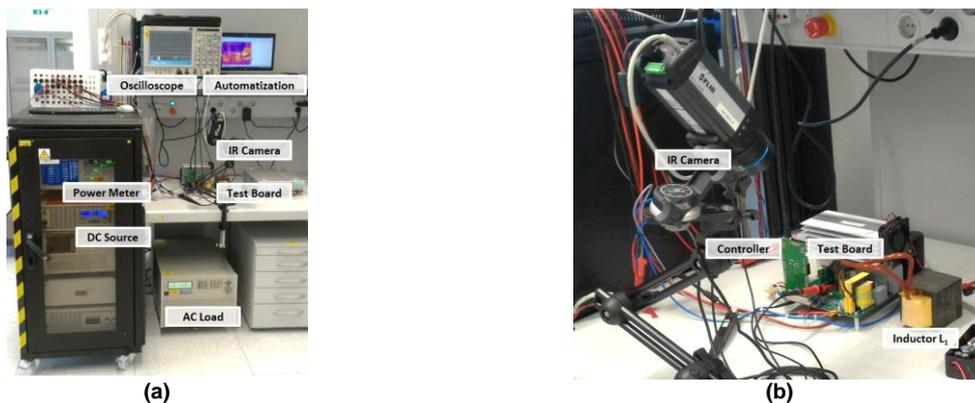
Figure 7: Fully automated test setup (a) including all laboratory equipment and (b) board close-up view
