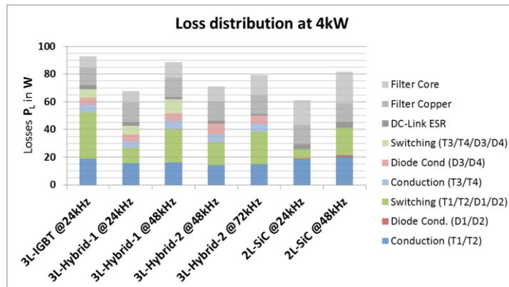
Figure 9: Estimated loss breakdown for the considered inverter solutions at  $\cos(\phi)=1$ .
