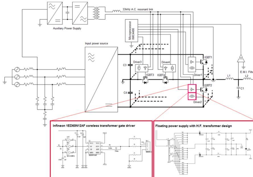
Figure 3 : Block diagram of the three-level T-Type inverter system. It is represented for a single-phase system. Details of the coreless transformer drivers and HF transformer are highlighted in the rectangles.
