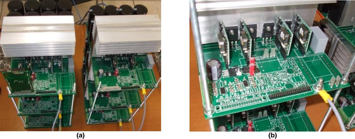
Figure 2: (a) Three-level three-phase T-Type system. Assembly phase of two three-phase systems and (b) close up view to the single-phase structure prior to assembling the EMI filters.
