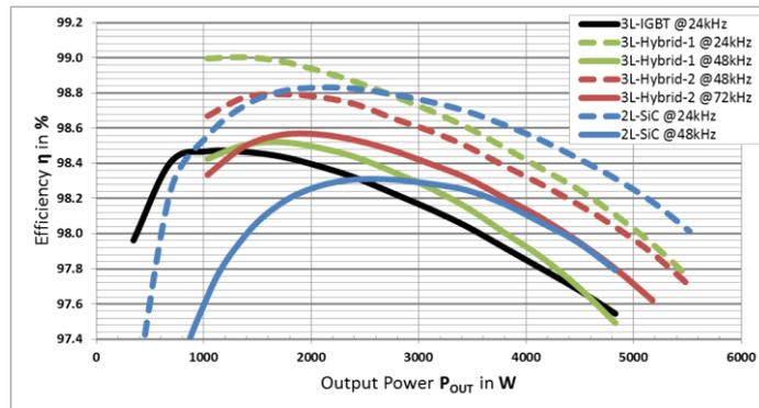
Figure 8: Measured efficiency comparison of the selected inverter solutions at  $\cos(\phi)=1$ .
