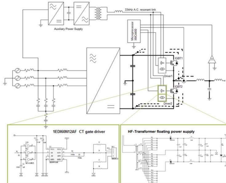
Figure 5: Block diagram of the two-level inverter system, sketched for a single-phase. Details of the coreless transformer and HF isolation transformer are indicated in the highlighted rectangles.
