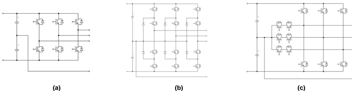
**Figure 1: most commonly used Inverter configurations: (a) two-level (B6, Six-Pack) Inverter; (b) three-level Neutral Point Clamping Diodes (NPC-1) Inverter; (c) three-level transistor clamped (T-Type) Inverter;**
