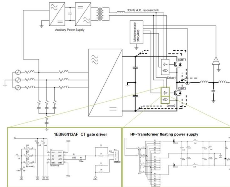
Figure 2: Block diagram of the two-level inverter system, sketched for a single-phase. Details of the coreless transformer and HF isolation transformer are indicated in the highlighted rectangles.
