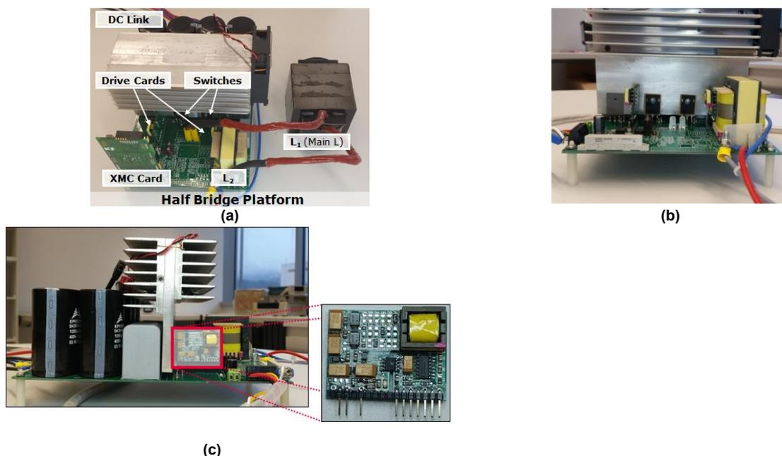
Figure 1: (a) close up view of a single-phase unit with short description of the main subsystems, (b) front view of the single-phase unit, (c) side view of the single-phase unit with a close-up view of a gate driver daughter board.
